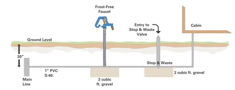
Use only 1" Schedule 40 PVC from main line to cabin with stop and waste valve near cabin.
